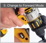
Ensure the drill is in Forward mode otherwise the auger will just spin on the surface. It is marked with a forward arrow or the letter 'F'.
