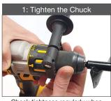
Check tightness regularly when digging to avoid stripping the head. With metal chucks, you can lock it by one click backwards after fully tightening.
